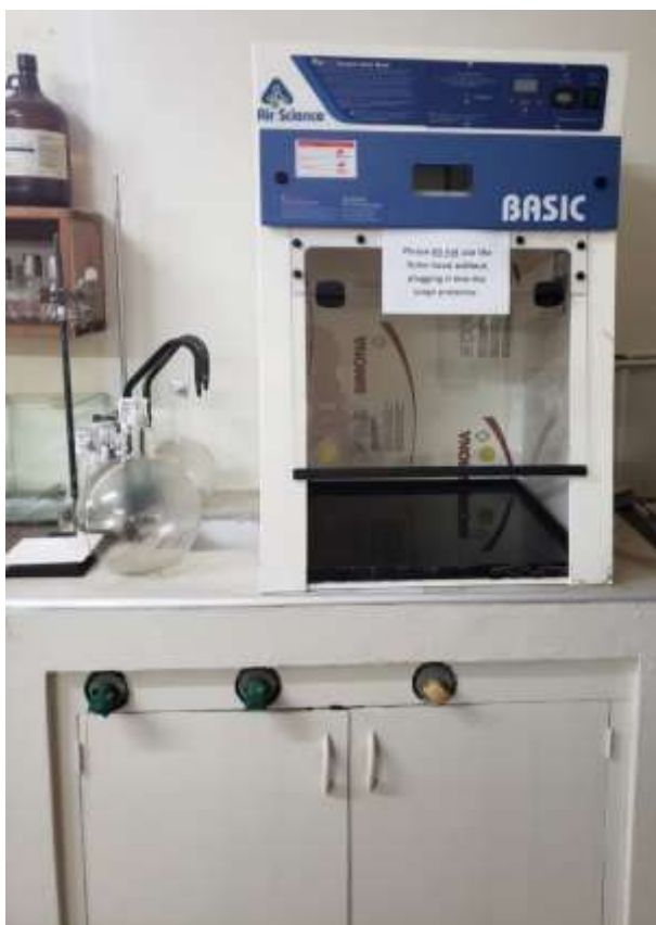
Portable (ductless) fume hood set up in Lab 6, Block B, UWI (Mona).
