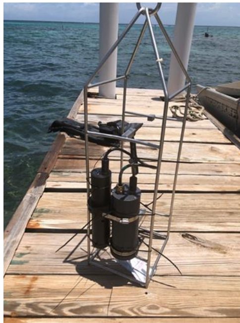
Images: Preparing the iSAMI and CTD sensors for deployment by Dr Camilo Trench, Shanna-Lee Thomas (left) (Photo Credits: Marcia Ford). The iSAMI and CTD sensors on the dock ready for deployment (left) (Photo Credits: Marcia Ford)
