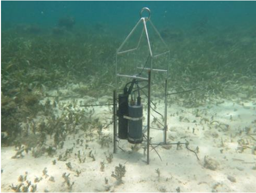
Images: The iSAMI and CTD sensors deployed in the back reef at Discovery Bay, Jamaica (left) (Photo Credit: A. Johnson) by deployment team Anthony Johnson and Oneil Holder (right).
