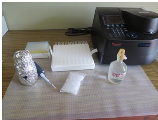
Images: Lab equipment for total alkalinity titrations (left) and spectrophotometric pH analysis (right). (Photo Credits: Marcia Ford).
