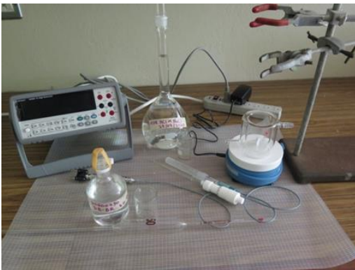
Images: Lab equipment for total alkalinity titrations (left) and spectrophotometric pH analysis (right). (Photo Credits: Marcia Ford).
